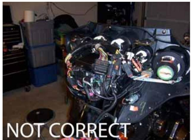
6. Make sure fast harness is tie wrapped out of the way prior to replacing fairing check to make sure you have proper clearance **DO NOT!!!!** Force fairing back into place. Always check your HD Manuel for proper torque settings.
